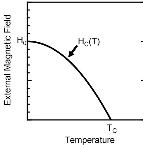
Coexistence curve between superconducting and normal phase.
